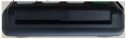
Inspect the MSR card slot to make sure that no any additional card reader and other
