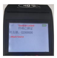
If the device is tampered state, the user must contact the device maintenance personnel immediately for help.
