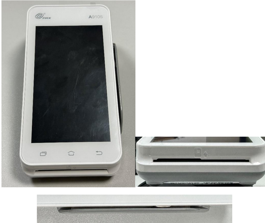
Figure 1-2 PAX A910S 5-inch Appearance(fourth last character of the hardware version number is 0 or 2)
