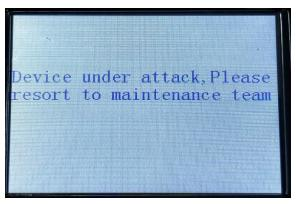
If the device detects tamper event, it will clear the key used to protect other key within the device immediately, and then restart automatically.
