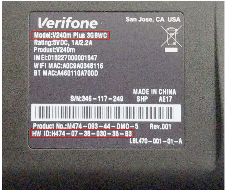
Figure 3, Hardware Identification via Product ID label
