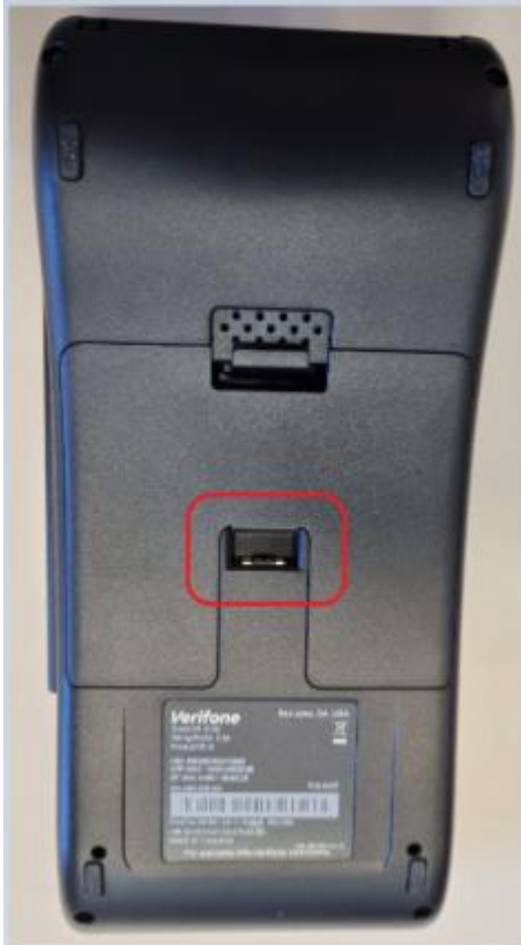
Example of a docking port on the back of a V210 4G series device
