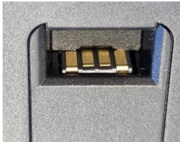
Example of a docking port on the back of a V210 4G series device
