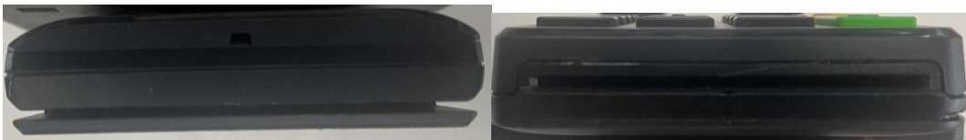
Figure 6 – MP35 MSR and ICC card slot
