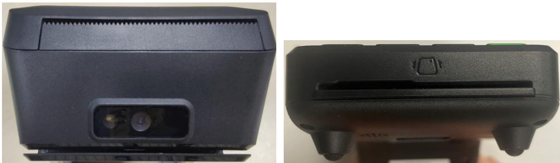
Figure 7 – MP35P MSR and ICC card slot
