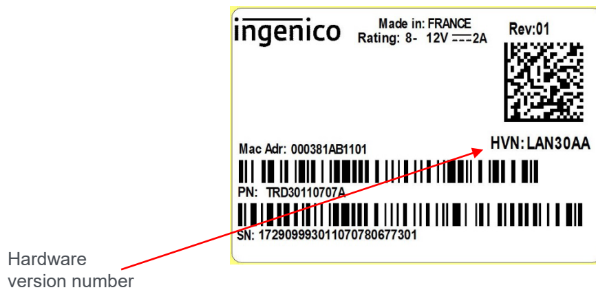
Figure 5 – Lane/3000 or Desk/1500 product hardware identification
