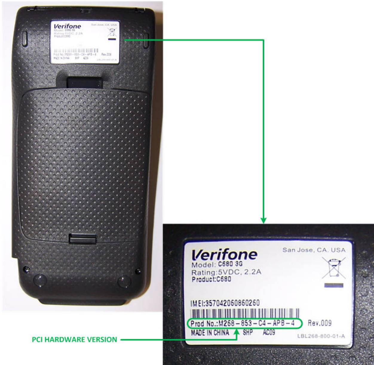
Figure 2, Match the PCI Hardware Version listed on the device
