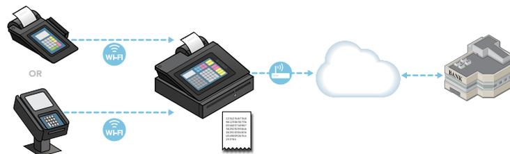
A **PAYMENT SYSTEM** includes the entire process for accepting card payments. Also called the cardholder data environment (CDE), your payment system may include a payment terminal, an electronic cash register, other devices or systems connected to a payment terminal (for example, Wi-Fi for connectivity or a PC used for inventory), and the connections out to a merchant bank. It is important to use only secure payment terminals and solutions to support your payment system.
