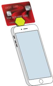
You accept payments via a PCI-listed SCR (Secure Card Reader) attached to a mobile device
